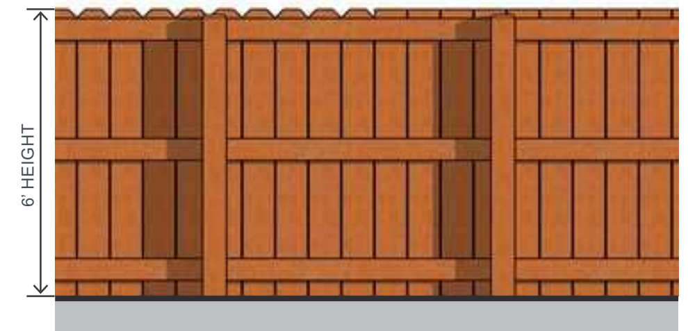
6' PRIVACY FENCE WITH VERTICAL PICKETS (ORIENTATION TO BE DETERMINED BY BUILDER OR HOMEOWNER.)
